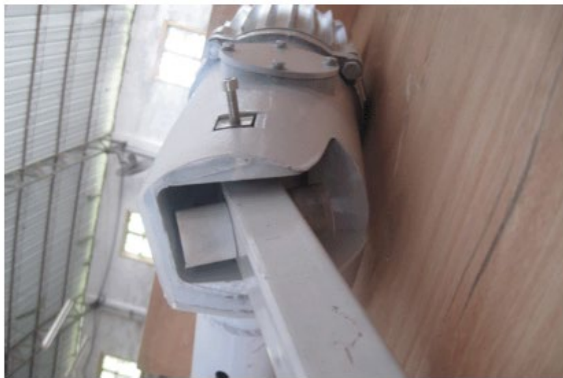
5.5 Fix the tail vane by M10 screws, washers.
